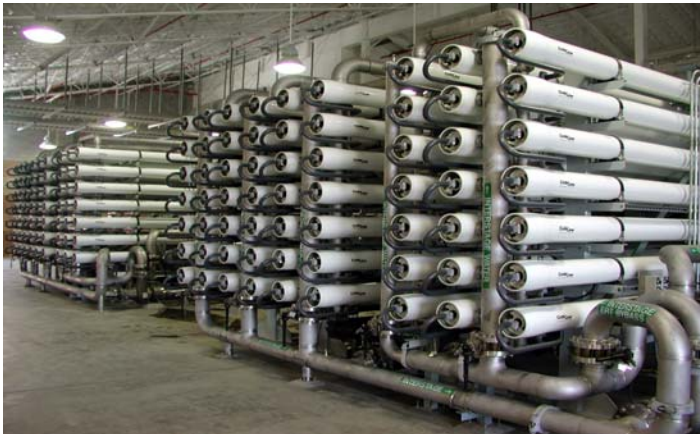
Desalination uses Reverse Osmosis
